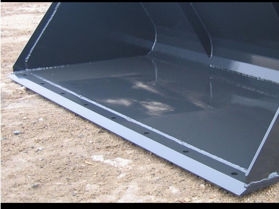
The Granular Material Bucket has more rollback to minimize spillage of material
